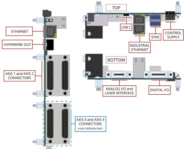
Figure 1-3: iXI4-OEM Transconductance Amplifier Controller
