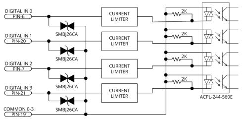
Each group of four inputs must be connected in an all sourcing or all sinking configuration. **Figure 2-25: Digital Inputs Connected to Current Sourcing (PNP) Devices**
