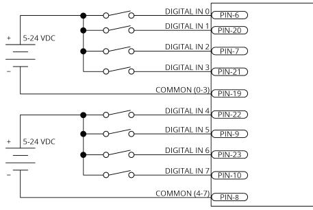
Figure 2-26: Digital Inputs Connected to Current Sinking (NPN) Devices
