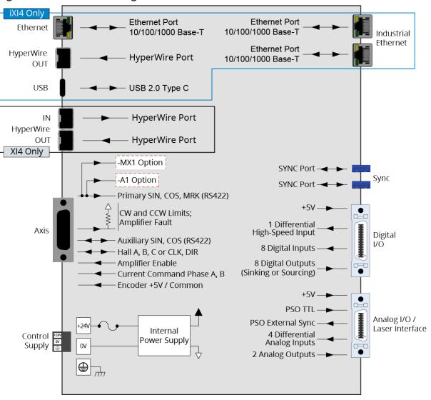
Figure 1-5: Functional Diagram
