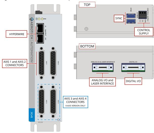
Figure 1-2: XI4 Transconductance Amplifier Controller
