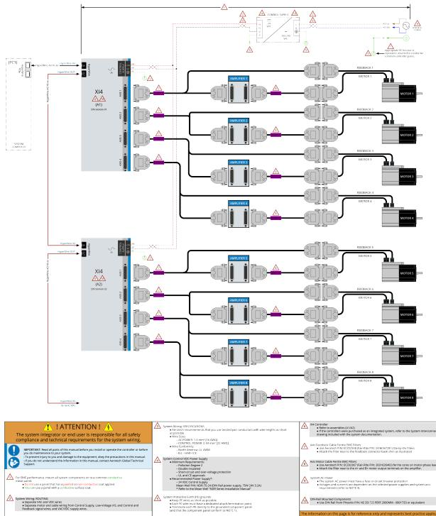
Figure 2-33: PC-Based Controller System Interconnection (Best Practice)
