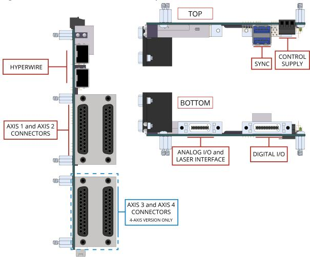
Figure 1-4: XI4-OEM Transconductance Amplifier Controller
