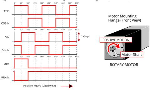
Figure 2-17: Encoder Phasing Reference Diagram (Standard)
