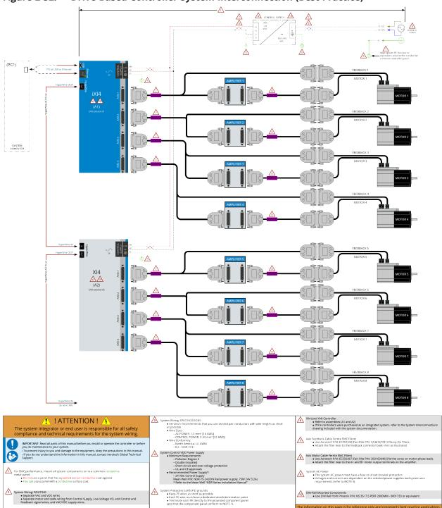
Figure 2-32: Drive-Based Controller System Interconnection (Best Practice)
