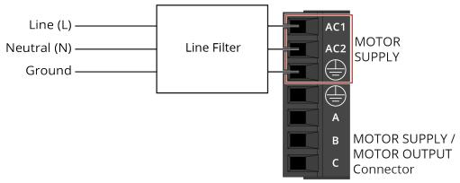
**Table 2-3: Motor Supply Connector Wiring Specifications**
