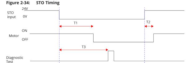
The software is typically configured to execute a controlled stop when the STO state is first detected. If power is reapplied to the STO inputs before the STO Delay Time, an STO hardware shutdown will not occur but a software stop may, depending on the width of the STO pulse. The controller will ignore STO active pulses shorter in length than the STOPulseFilter parameter setting.
