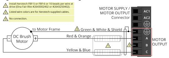
Table 2-11: Wire Colors for Aerotech-Supplied DC Brush Motor Cables
