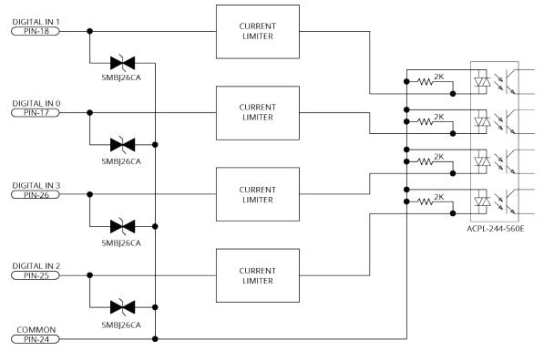
Figure 2-44: Digital Inputs Connected to Current Sourcing Devices
