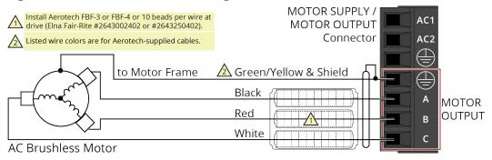
Table 2-9: Wire Colors for Aerotech-Supplied Brushless Motor Cables
