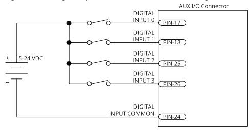
Figure 2-45: Digital Inputs Connected to Current Sinking Devices
