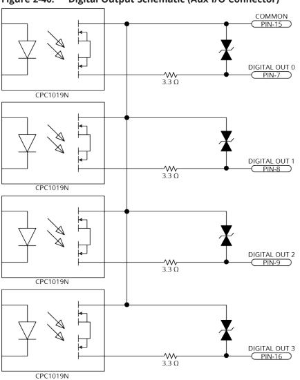
Figure 2-40: Digital Output Schematic (Aux I/O Connector)
