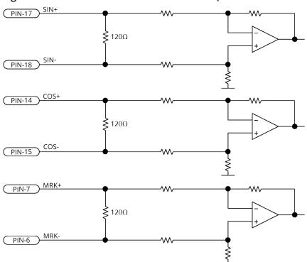
Figure 2-23: Sine Wave Encoder Schematic (Feedback Connector)
