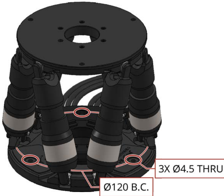
Figure 2-2: Mounting Hole Locations
