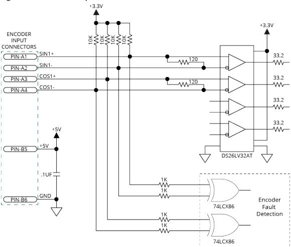
Figure 2-13: Encoder Input Connector Encoder Connections
