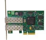
SFP ports for the glass optical fiber, highspeed HyperWire communication bus and can connect up to 32 axes of precision motor drives — each capable of operating at industryleading performance levels.
